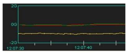
When then vehicle is static or "at rest" the lines will be nearly horizontal or charted in a straight line, with no deflection or charted deviation. Note the Z-axis charting is not at "0" as the vehicle is subject to gravity so there is a built in baseline at "1G" as long as the vehicle remains on planet Earth, caused by the forces of Earths gravity thus a permanent deflection baseline.
