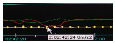
"Z" axis deflections can indicate sudden changes in up or down inertia, that can be caused by hitting large potholes, running over curbs or running over speed bumps at a high rate of speed. Anything that will cause the vehicle to drop down or bounce up will be reflected on the "Z" axis charting. Common problems include; school bus drivers who do not slow down
