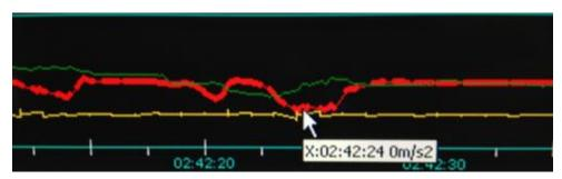
"X" axis chart deflections can indicate rapid acceleration and hard braking
