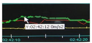
"Y" axis chart deflections can indicate high-speed hard turns, erratic lane changes and failure to maintain lane that cause vehicles to lean hard to their sides. High Speed Turns can cause vehicles with a high center of gravity to flip or roll over endangering driver /passenger lives and damaging property.
